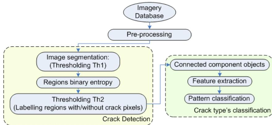
Figure 2: Automatic crack detection and type's classification system architecture.
