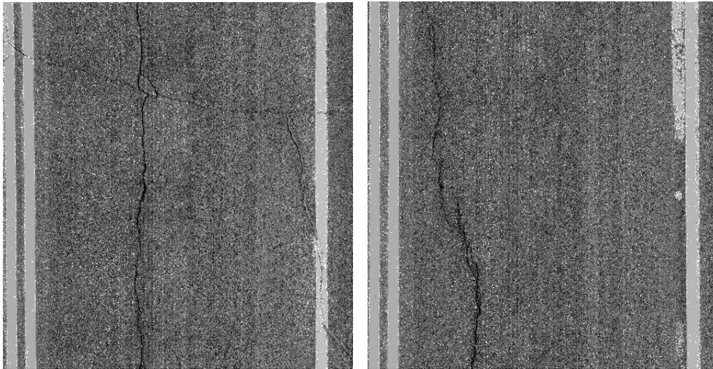
Figure 1: LRIS crack images with dimensions of 4015 x 3786 pixels, showing the entire lane.
