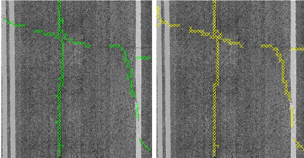
Figure 3: Experimental crack region detection result (left) and the respective ground truth data (right), for the left image show in Figure 1.
