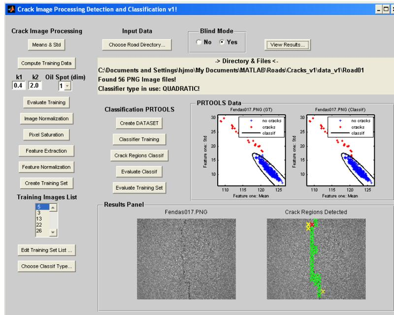
Figure 4: Graphical user interface of the automatic road surface imagery analysis software developed.
