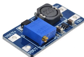
Figura 5.7: Módulo de Step-Up MT3608 (em https://www.botnroll.com/pt/step-up/3652-mt3608-conversor-dc-dc-step-up-sa-da-max-28v-2a.html ).
