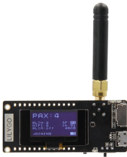
Figura 5.1: LILYGO TTGO T3 LoRa32 868MHz V1.6.1 [LIL24].
